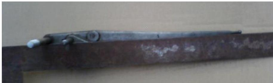
(13) Put a straight edge against the bolts. The straight edge MUST BE ON THE BACKSIDE OF THE CONTROL ARM (see the picture). If you put the straight edge on the wrong side of the bolts, you will not get the correct shape to the control arm.
