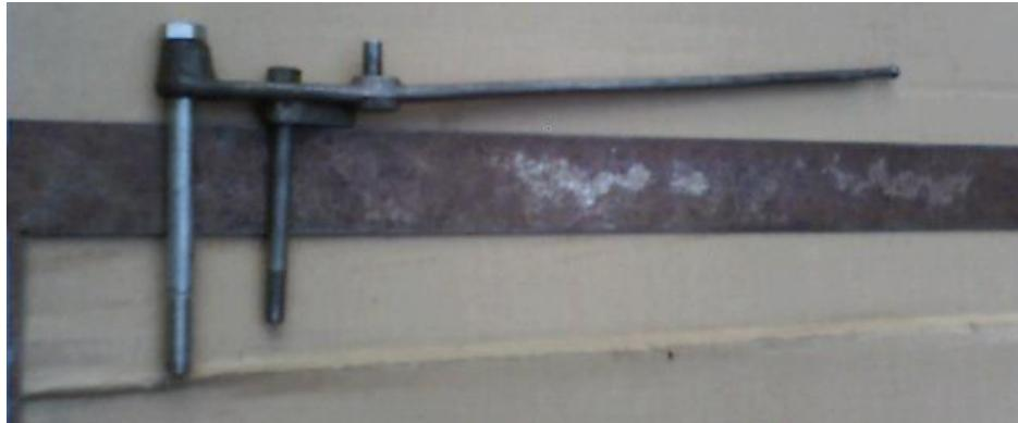
(12) Put a 1/2 inch bolt in the end hole of the control arm. Put a 3/8 inch bolt in the next hole. Note: the control arm has a bend to the side; do NOT straighten out this bend (see picture).
