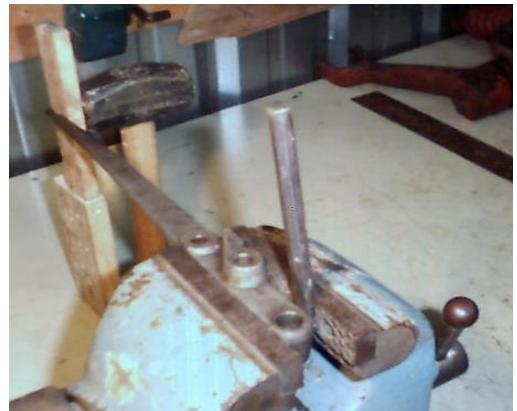
(17) Continue to hammer on the control arm until it aligns correctly as described in step (14) above.
